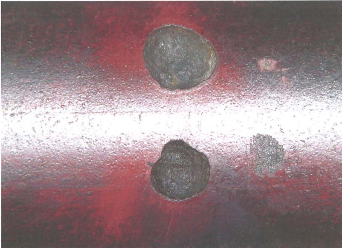
Figure 21 External Pits on the Gas Lift Mandrel from 4,100 Feet
