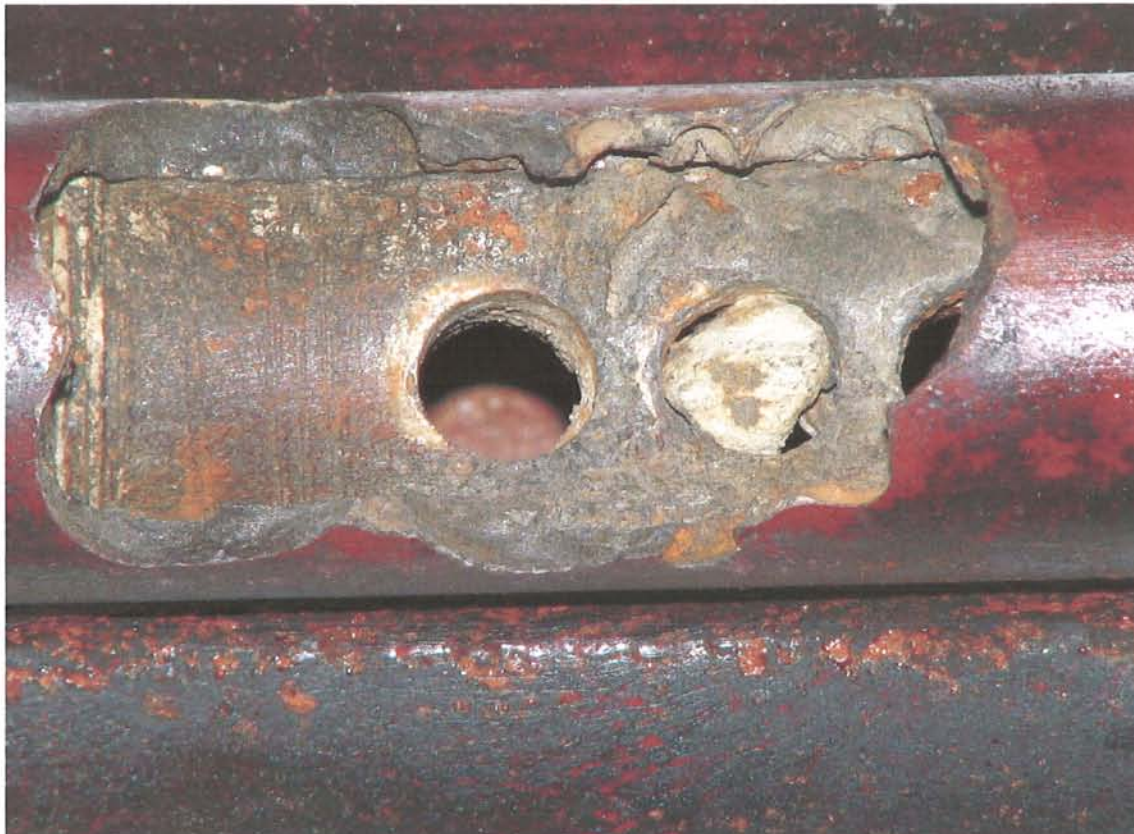
Figure 23 External Corrosion on the Gas Lift Mandrel After Cleaning
