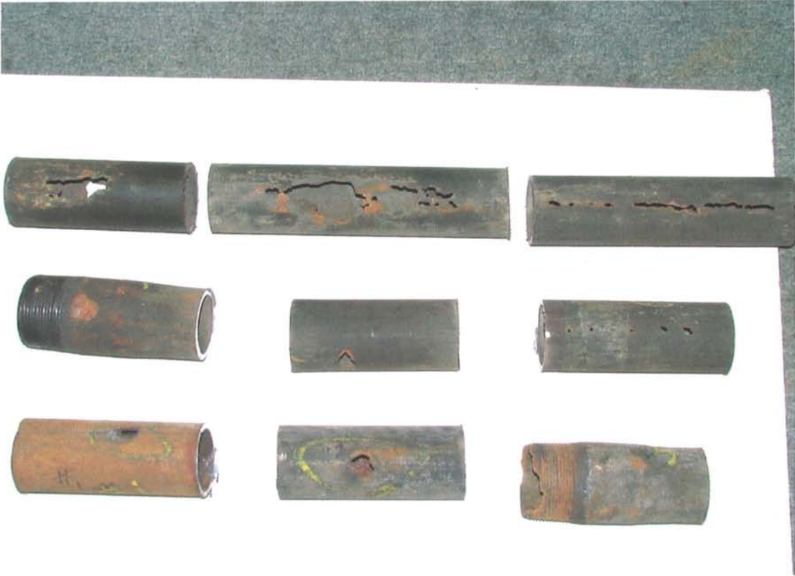
Figure 1 Sections of the Tubing Received for Examination
