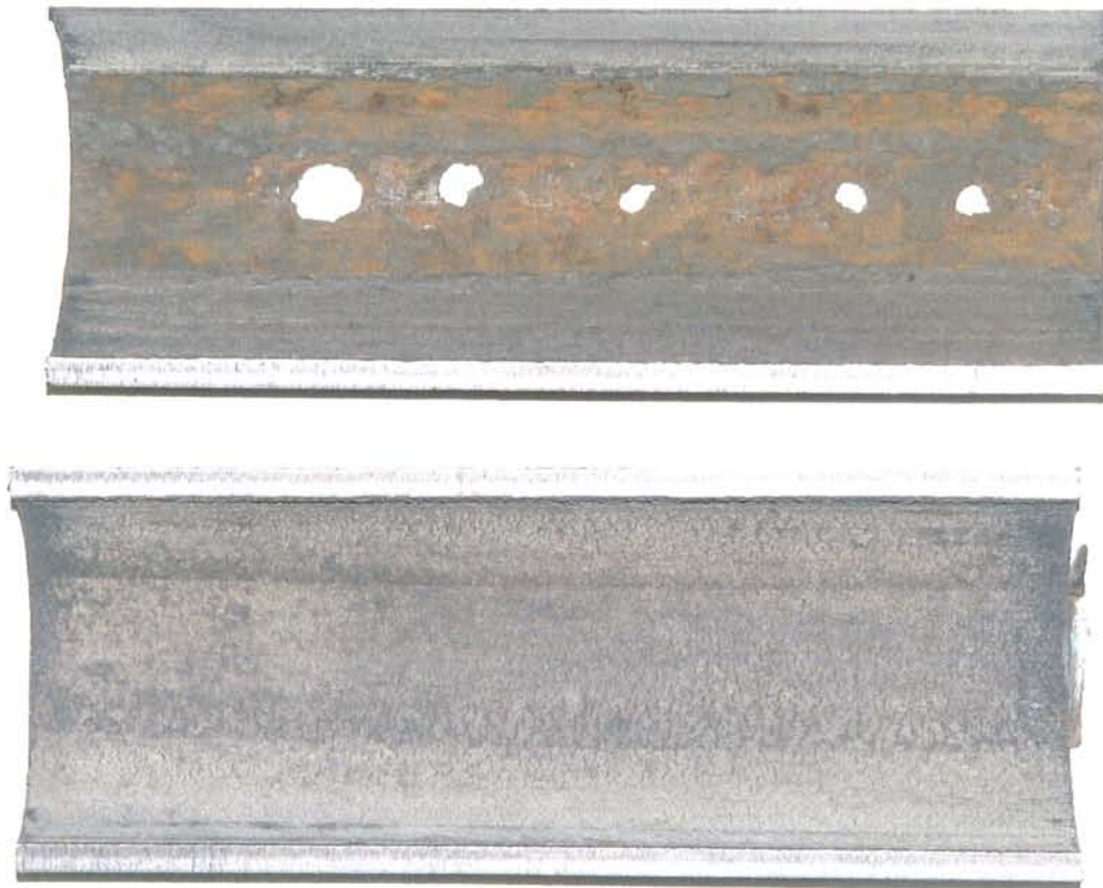
Figure 13 Internal Surface of Section #6 After Cleaning
