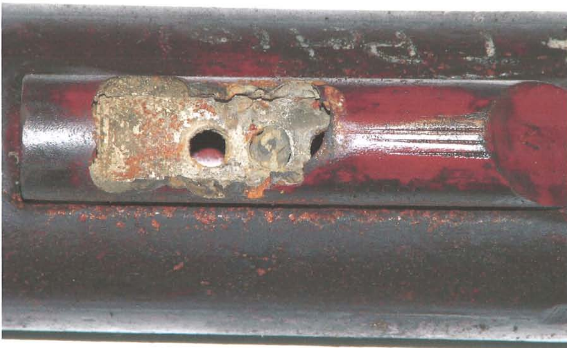
Figure 22 External Corrosion on the Gas Lift Mandrel from 4,100 Feet
